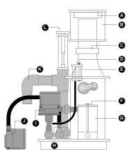
B. Collection cup C. Twist-lock fitting (Bayonet) D. Air intake tap E. Air intake silencer
